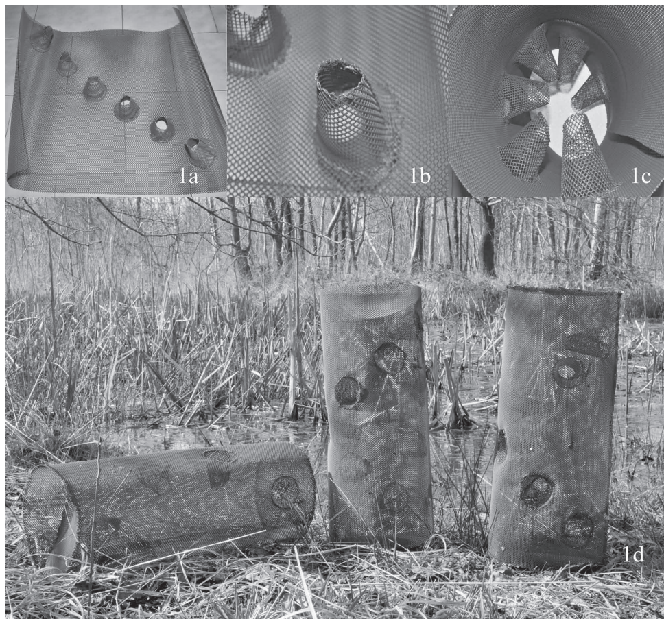
Figure 1. Construction phases of each trap used in this study: (a) six funnels were sewn to along the diagonal; (b) detail of a single funnel; (c) each trap was bent over and the edges were sewn together with iron wire; (d) three of the traps in the field. The trap can be placed either horizontally or vertically.
